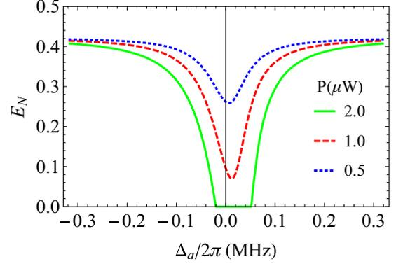
FIG. 8. (Color online) Plots of the logarithmic negativity  $E_N$  vs the detuning  $\Delta_a$  for the thermal bath temperature of the first resonator  $T_c = 50 \text{ mK}$  and for the thermal bath temperature of the second resonator  $T_a = 100 \text{ mK}$  and for different values of the microwave drive pump power  $P = 0.5 \mu\text{W}$  (dotted blue curve),  $1.0 \mu\text{W}$  (dashed red curve), and  $2.0 \mu\text{W}$  (solid green curve). All other parameters are the same as in Fig. 2.
