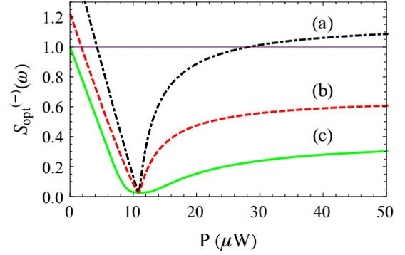
FIG. 5. (Color online) Plots of the squeezing spectrum vs the microwave drive pump power  $P$  ( $\mu\text{W}$ ) for the bath temperature of the first resonator  $T_c = 2$  K, the membrane's bath temperature,  $T_b = 10$  mK, and for different values of the bath temperature  $T_a$  of the second resonator: (a)  $T_a = 250$  mK (dot-dashed black curve), (b)  $T_a = 150$  mK (dashed red curve), and (c)  $T_a = 50$  mK (solid green curve). All other parameters are the same as in Fig. 2.
